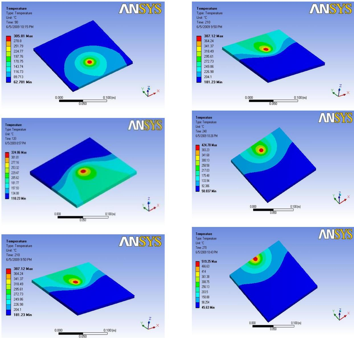
Fig.5. A View of temperature maps of the Al606-T6 alloy of 30s, 60s, 90s, 120s, 150s, 180s, 210s, and 240s of welding (steady state conditions) using the ANSYS model with  $af=0.4$  and  $q=0.1$
