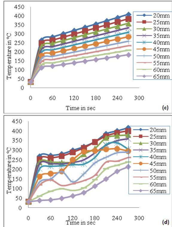
**Fig.6 Stir welding temperature as a function of welding time at varies distance weld area of (a)Advanced side(Experimental), (b) Retreating side(Experimental), (c)Advanced side(Numerical) and (d) Retreating side(Numerical)**
