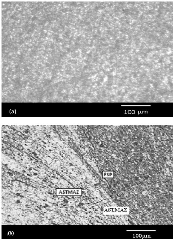
Fig. 8. Optical Micrograph of Al6061-T6 Alloy and Welded area
