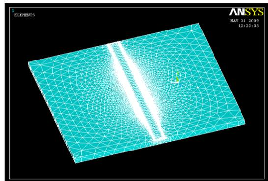
Fig. 4. A view of Finite Element mesh of Friction stir welding plate
