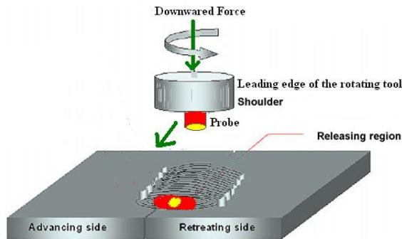
Fig. 1. A schematic representation of the Friction stir welding process
