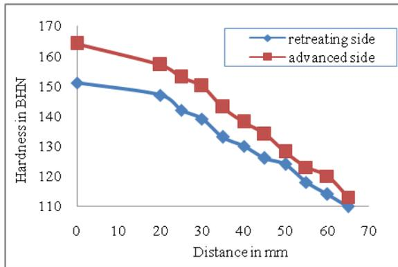
Fig.7. Hardness of Al6061-T6 alloy from weld area
